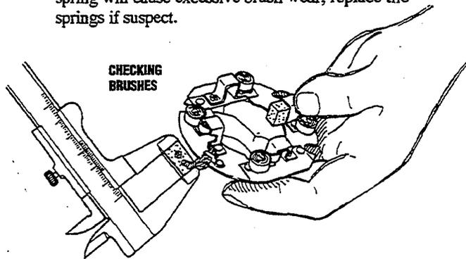
3. Check for insulation between the positive brush holder and holder base. If poorly insulated, replace the holder assembly. Also check the brush holders for proper staking.
