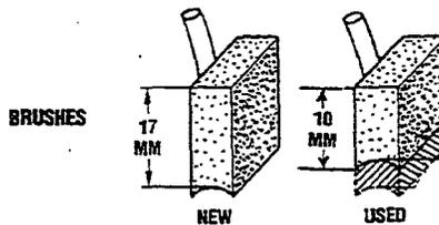
2. Check the brush spring tension. A weak or defective spring will cause excessive brush wear; replace the springs if suspect.
