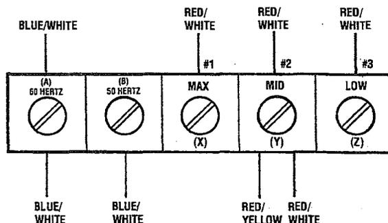
**NOTE:** On some units A and B may be reversed. To ensure a proper connection, be sure the blue & white striped leads coming off A or B go to the numbered terminal stud on the AC terminal block — #5 for 60 hertz and #6 for 50 hertz.
