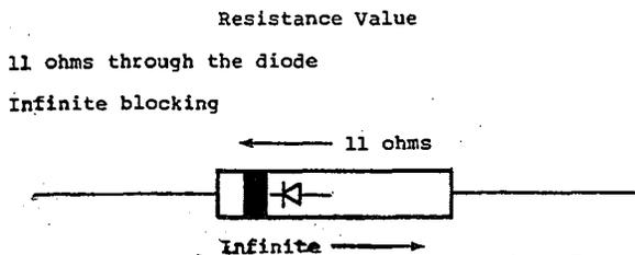
The diodes can be easily checked in place with the use of a common automotive 12-volt high beam headlight bulb, some jumper leads and the generator's 12 volt starting battery.
