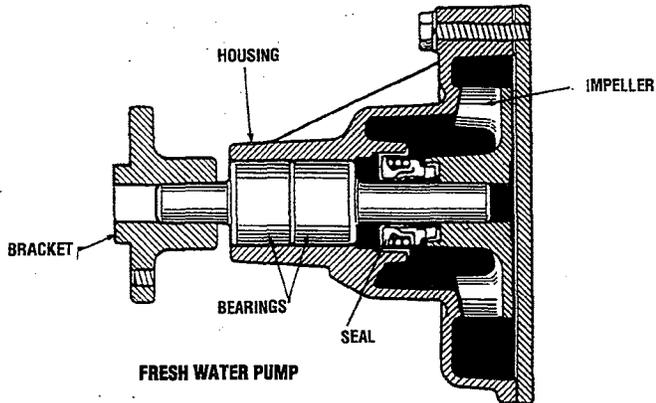
*The water pump* is a centrifugal impeller type and is mounted on the front upper part of the cylinder block. The pump shaft is supported on maintenance-free (grease-filled) double-row radial ball bearings.
