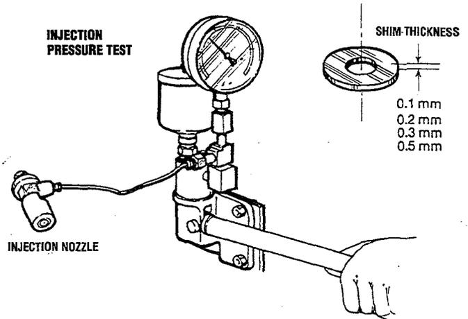
2. **Chattering Test.** For the chattering test, operate the tester lever slowly. If the nozzle sprays sharply and intermittently, the nozzle is considered good. The nozzle should spray fuel straight in its axial direction. A nozzle is defective if it sprays fuel in a wrong direction or in several separate strips. Also a spray in the form of particles indicates a defect. These defects may sometimes be caused by clogging with dust, therefore all parts should be carefully cleaned before assembly.
