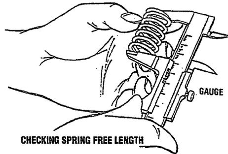
3. Check the squareness of each spring. Replace the spring if it tilts excessively.
