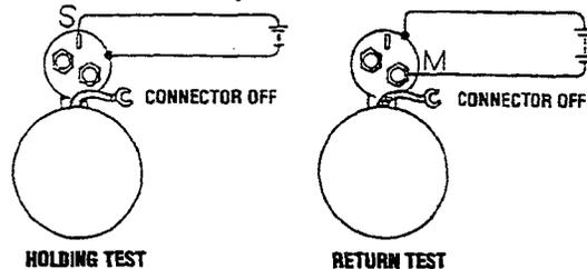
4. **Return test.** With a battery connected to the solenoid terminal "M" and to the starter body, manually pull out the pinion fully. The pinion must return to its original position when released from being held by hand.
