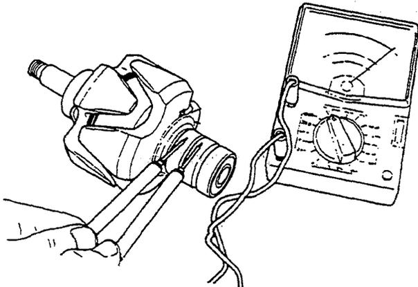
Check for continuity between the slip ring and the core. If there is continuity, it means that the coil or slip ring is grounded. Replace the rotor assembly.
