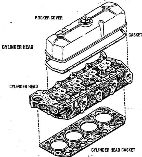
The cylinder head gasket is made of carbon graphite. It is provided with stainless steel sheet grommets around the bores for improved heat and pressure resistance. The gasket requires no sealant when assembled.
