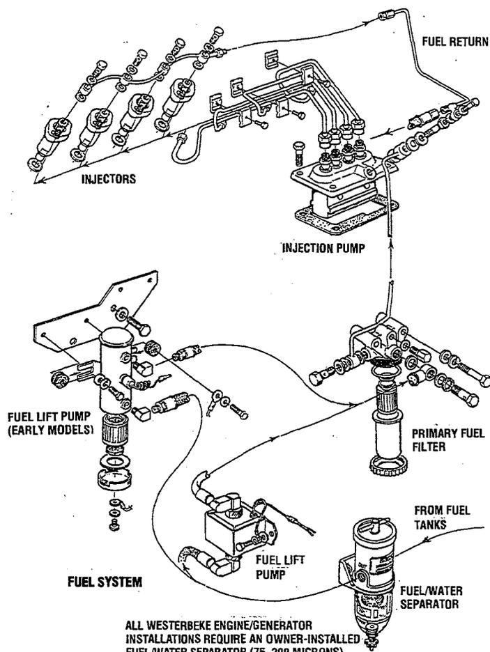
ALL WESTERBEKE ENGINE/GENERATOR INSTALLATIONS REQUIRE AN OWNER-INSTALLED FUEL/WATER SEPARATOR (75–200 MICRONS)
