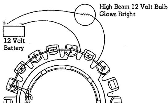
**Reverse the leads across the diode.** The diode should block voltage passing through it, and the headlight should not glow, or it may glow faintly.
