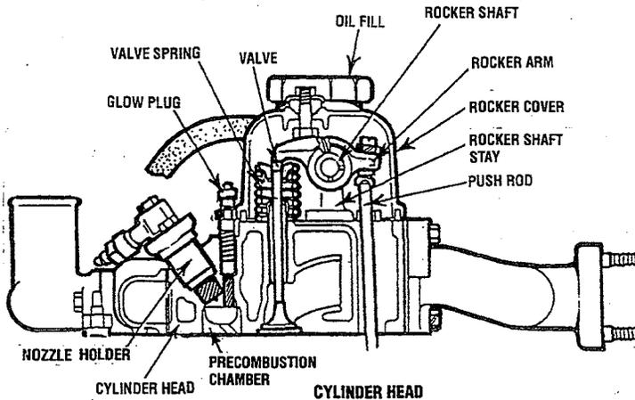
The precombustion chamber is of a swirl chamber type (Ricardo) made of heat resisting steel and is press fitted in the cylinder head. This chamber, therefore, requires no disassembly.
