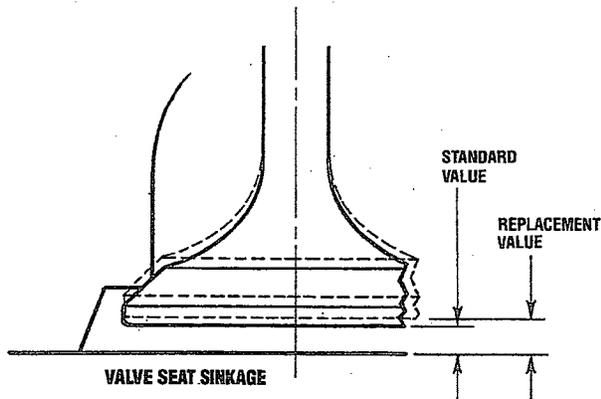
4. Check the valve seat inserts if provided, for proper fit. Replace any that fit loosely.
