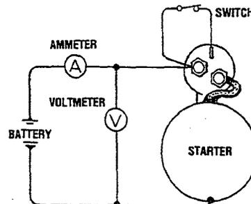
**CAUTION:** Use thick wires as much as possible and tighten every terminal securely. This is a solenoid shift-type starter which makes a rotating sound louder than that of a direct-drive type starter. When detecting starter rotation at the pinion tip, be careful not to come in contact with the pinion gear when it protrudes.
