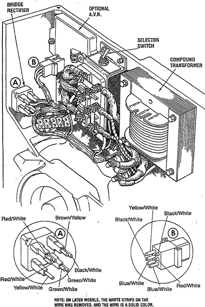
**NOTE:** There should be no continuity found between any of the lifted stator leads and the case ground. Also, no continuity should be found between the connections of the two groups.
