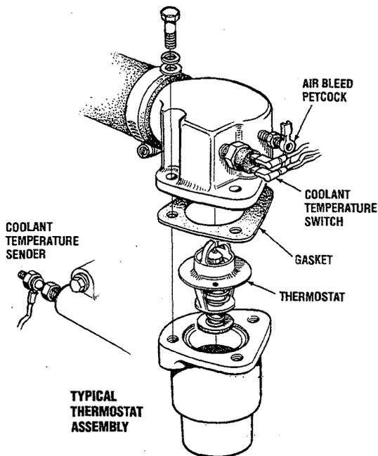
*Thermostat.* A thermostat housing is located on the cylinder head water outlet. Enclosed is a wax pellet-type thermostat. The valve opening temperature is not affected by variations of pressure in the cooling water passages.
